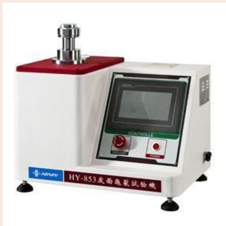
Use: for leather or fur particle surface elongation and cracking strength, or shoe material toe surface deformation resistance test. Complies with the following standards: ISO 3379, ISO 17695, QB3812.7, QB/T2712, GB/T 3903.40-2008, BS3144, BS3424, NFG52, DIN53325, IUP9, SLP9, SATRA TM24, DIN 53325, and Adidas GE-22.
